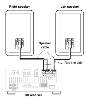
Remove the precut insulation from the ends of the speaker cables, and twist the bare wires tightly.
